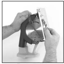
Fig 6. Installing blade.
